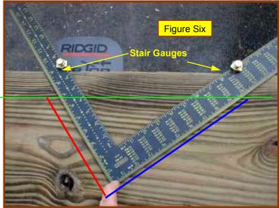
tread depth of the step above and/or below the one that is out of line. The red line represents a riser height. The blue line is a tread. Are you having trouble visualizing this? If so, check out
