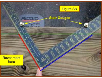
could then draw a line up the outside of the tongue and create your **second** riser. This is exactly what Figure Six above is showing you.
